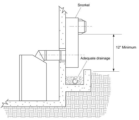
Figure 10 - Snorkel Termination with Drainage Pipe
